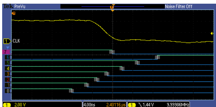
Figure 11: White edges indicate additional information is available by acquiring at a higher sample rate.
