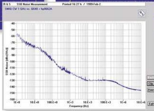
Typical SSB phase noise at f_c=1 GHz
