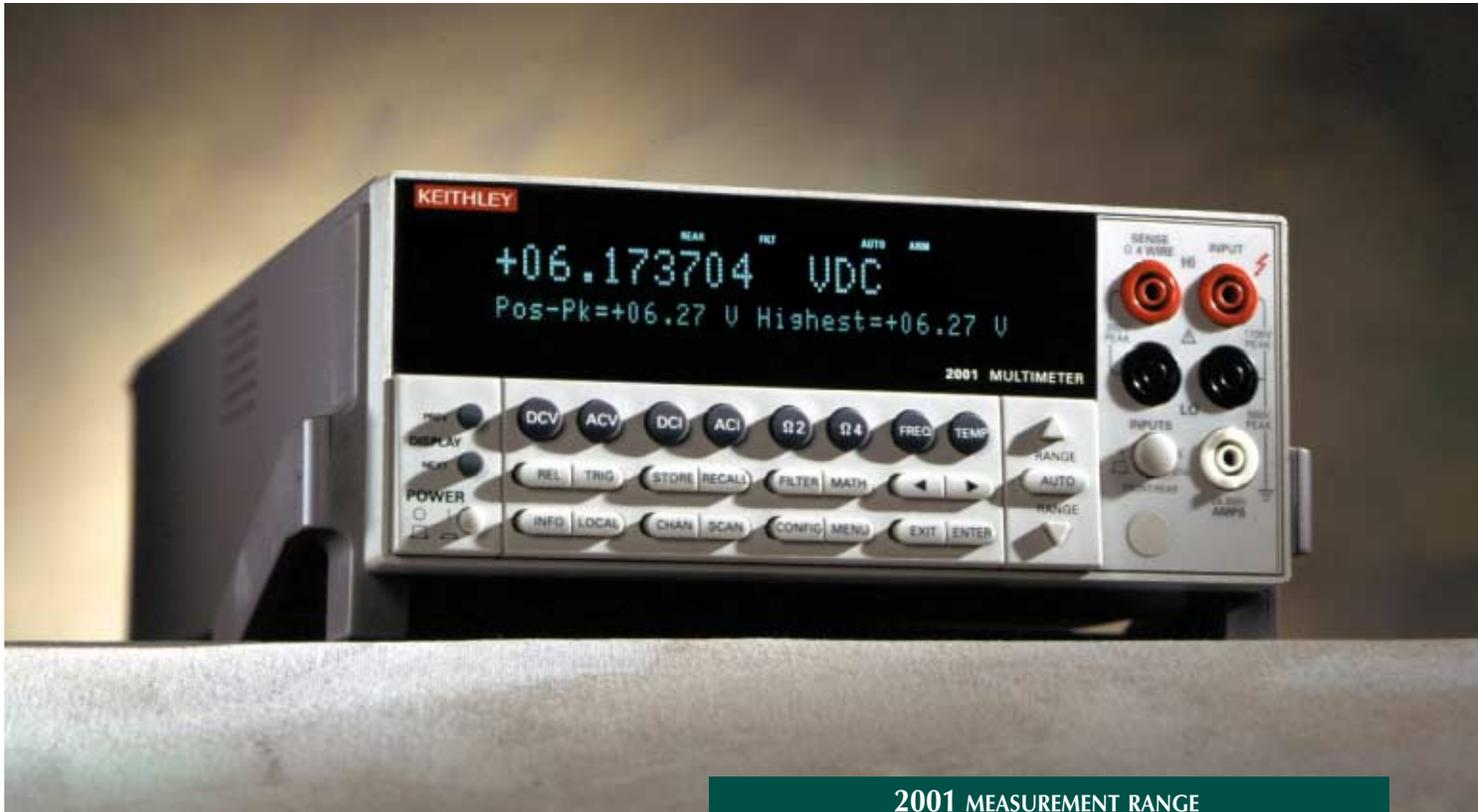
smaller changes. This high resolution also provides greater dynamic range, so it's possible to measure from 1µV to 20V on a single range and avoid range-shift errors.
