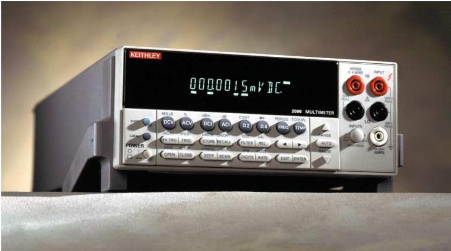
Using a precision, low-cost A-to-D converter enabled the Model 2000 design team to develop a unique error reduction algorithm. This algorithm corrects for drift errors associated with the resistor networks used for signal conditioning. Therefore, it allows the use of inexpensive resistor networks, while providing higher accuracy.
