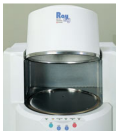
Large sample chamber allows samples to be analyzed without having to cut up the sample
