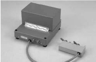
High Voltage BNC(f) connector for external bias input BNC(f) connector for voltage monitor output
